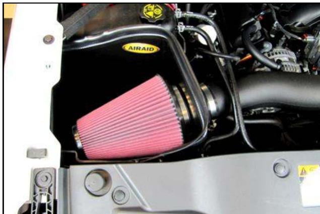
14. Install the Weather Strip onto the top edge of the Cold Air Box with the contour rolling away from the filter.
